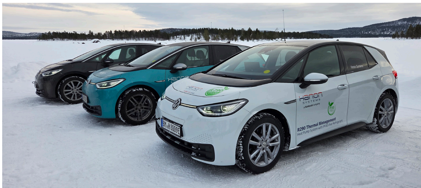
Figure 8-1: Test vehicles utilizing R290 and R744 thermal management systems perform real-world, cold climate testing in Finland
