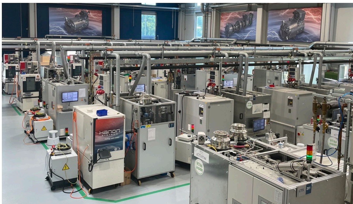
Figure 6-1: Test stands for natural refrigerant technologies at the Hanon Systems European Innovation Center in Kerpen, Germany
