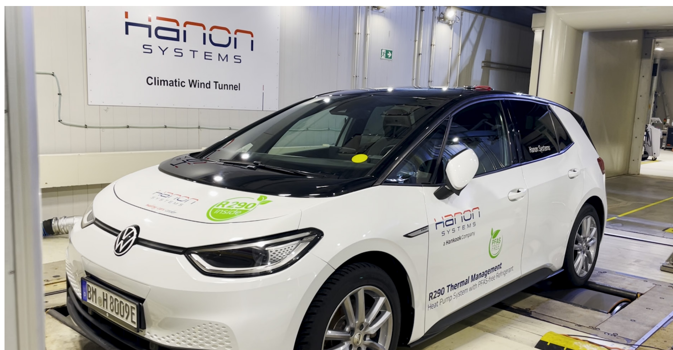
Figure 1-1: A test vehicle containing a thermal management system utilizing PFAS-free refrigerant sits inside the Hanon Systems European Innovation Center's climatic wind tunnel
